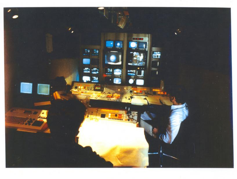
Some of the systems at JPL used to receive and process the real-time images and scientific date that the Voyager 2 spacecraft was sending back to Earth during its Neptune flyby on August 26, 1989.
