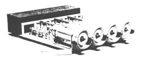
NASA-Lewis and its contractors are working on a bank of resistojet thrusters for the space station that will have a life goal of 10,000 hr while delivering 0.1-0.4 N of thrust.
