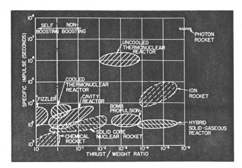
able material mixed in a solid "grain" with a moderating propellant, and "ignited" by removal of a control rod; often called a "fizzler".
