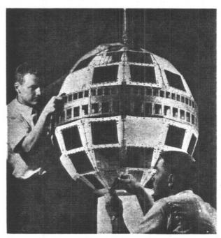
Communication satellites, such as this developmental model being worked on by Bell Telephone Labs technicians, represented a focus for the state of the art of both communications and instrumentation last year. At least three different experimental communication satellites will be launched next year.
