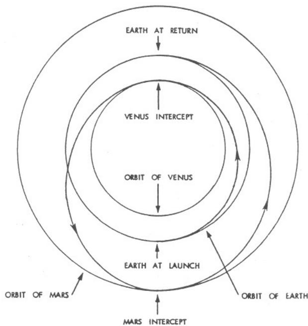
**Figure 6** Hohmann's rocket-propelled Earth-Venus-Mars-Earth multi-planet trajectory (1925).
