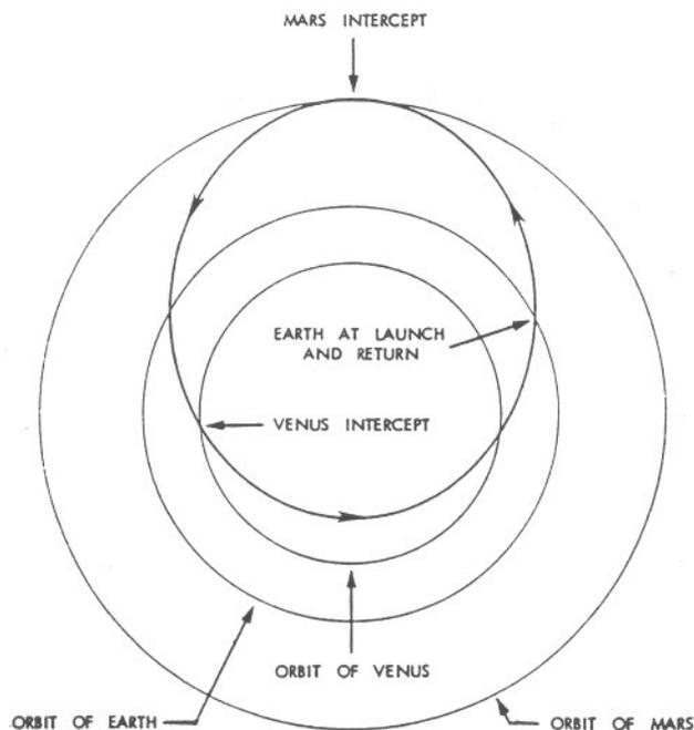
Figure 7 Crocco's constant elliptical path Earth-Mars-Venus-Earth multi-planet trajectory (1956).
