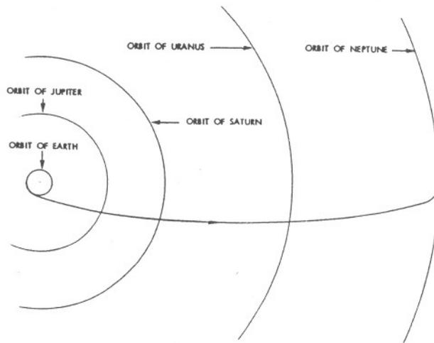
**Figure 2** Hohmann minimum-energy trajectory to Neptune
