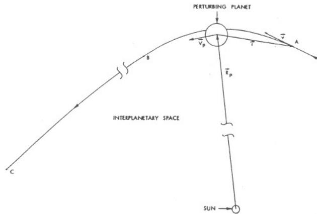
**Figure 4** Elements of the three-dimensional Restricted Three-Body Problem.
