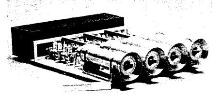
NASA-Lewis and its contractors are working on a bank of resistojet thrusters for the space station that will have a life goal of 10,000 hr while delivering 0.1-0.4 N of thrust. indications of an upturn. Apparent commitments to electric propulsion still face many hurdles and first full-blown applications are years down the road. Nonetheless, a number of decisions on electric propulsion do augur well for the technology.
